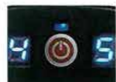
4. If the device is on and charging, the LED indicator on the device will be BLUE.
